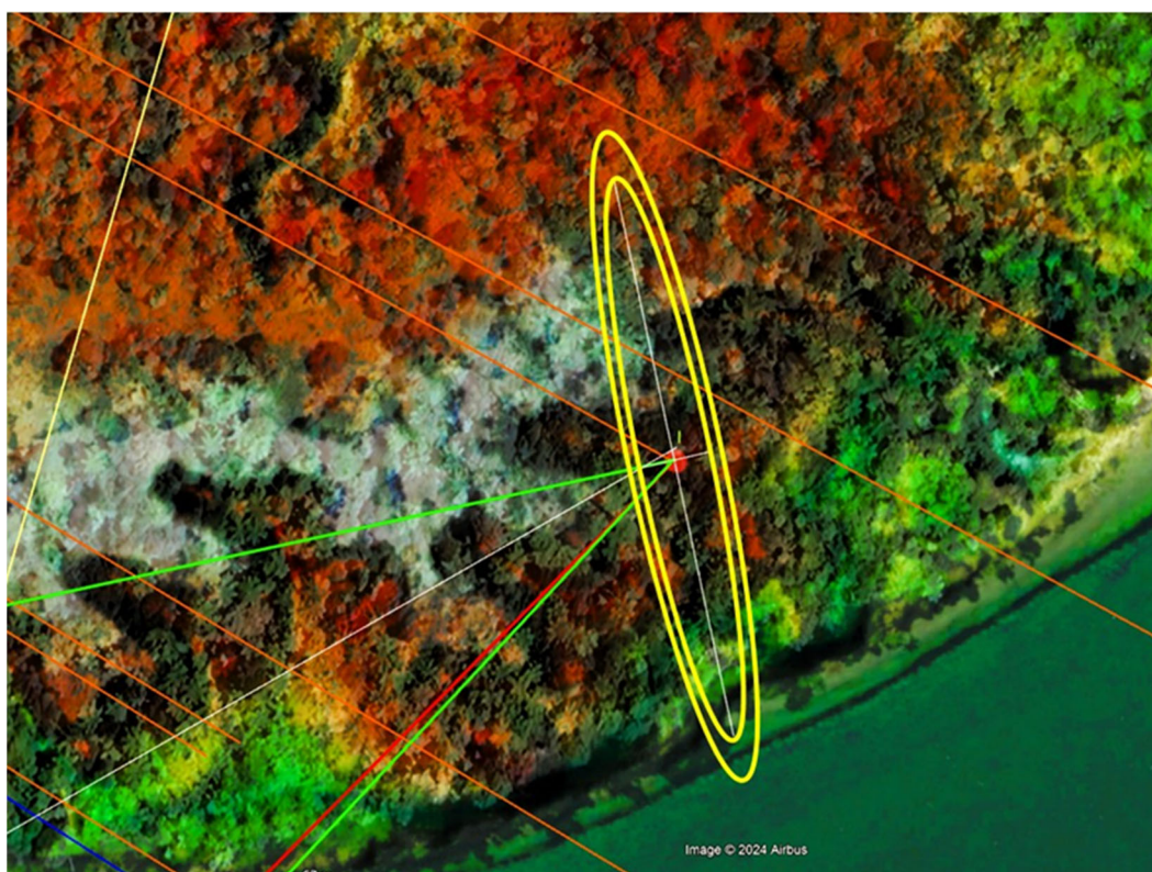
Figure 19. Error ellipses for Hochstetter's survey location of White Terrace. Inner ellipse for his two-minute compass. Outer ellipse for his 10-min compass. Coloured rays are survey bearings. (LiDAR courtesy of Adam Richardson at BOPLASS, Bunn).
