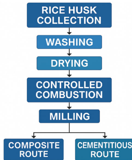
Figure 1. Processing Flow of RHA.
