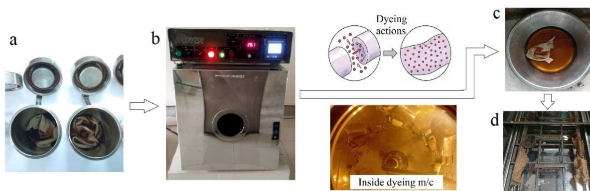
Figure 4. IR-assisted dyeing method, (a) Dye pot, (b) IR dyeing m/c, (c) washing after dyeing, and (d) curing.
